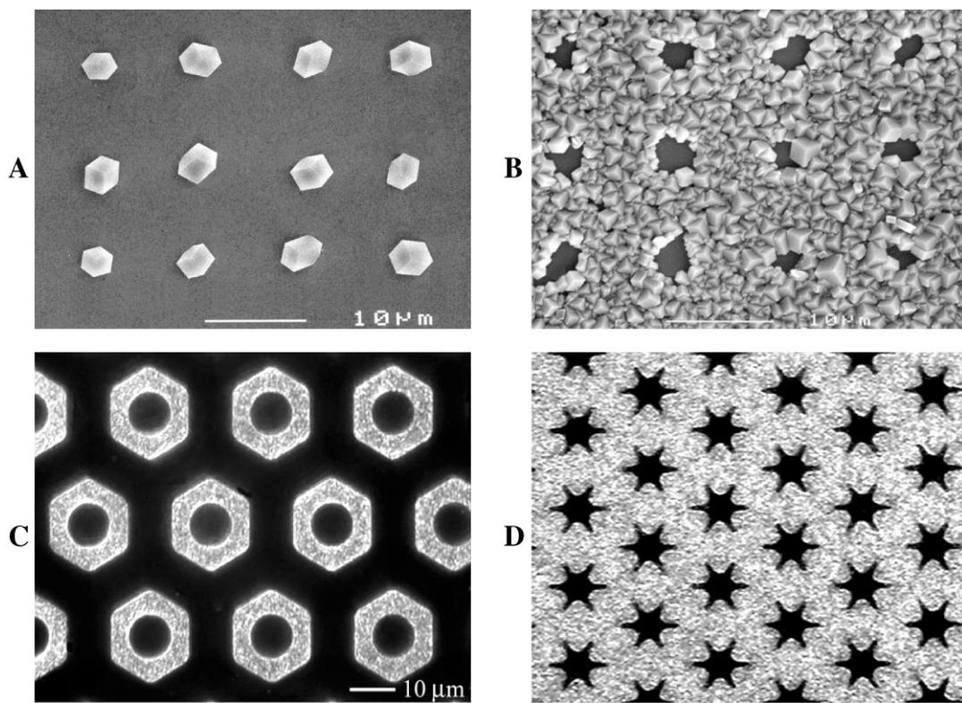
Fig. 4. Examples of high-resolution calcitic replicas of patterned SAMs (see text for details).
