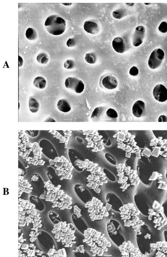
Fig. 1. Biogenic calcite crystals. (A) Convoluted shape of the spine of the brittle star *Ophiocoma wendtii*. (B) Epitaxial overgrowth of synthetic calcite crystals on the spine surface. Note that the nucleation of the newly formed calcite crystals occurred locally at specific sites on the surface.
