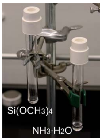
Fig. 1 Experimental setup for the exposure of samples to Si(OCH 3 ) 4 (TMOS) and NH 3 vapor, using NH 3 ·H 2 O solution. Samples were suspended from a wire within each of the two 25 mL test tubes.
