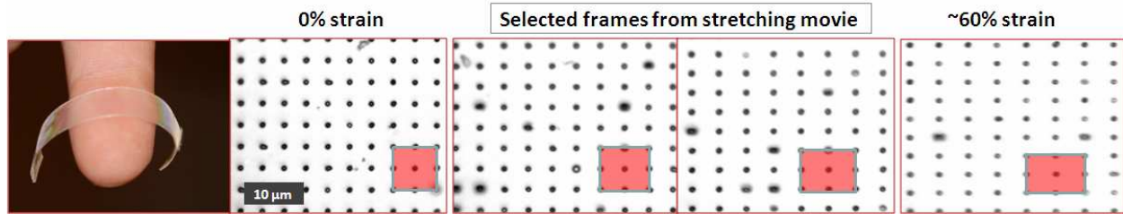
Figure 5. Mechanical in-plane actuation of micro/nanoscale rigid posts that are attached to a flexible, extendible elastomeric substrate, strained on a motorized stage. The sample is shown fitting the contour of the author's finger at left.
