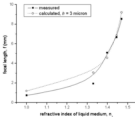
**Figure 6.** Measured and calculated focal lengths of microlens arrays versus the refractive index of the surrounding medium. The lines are used to guide the eye.
