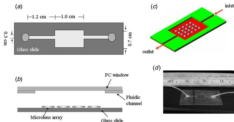
**Figure 2.** Design and dimensions of the fluidic channel integrated with microlens arrays. Illustrative images: (a) top view, (b) side view and (c) 3D view. (d) Actual image of the fluidic channel device used in the experiment.
