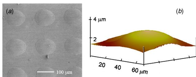
**Figure 4.** SEM and AFM images of the molded microlenses.
