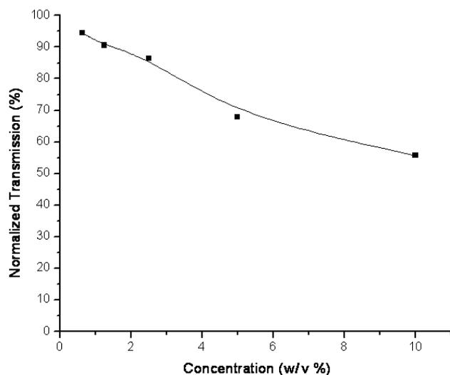
**Figure 7.** Transmission versus the concentration of congo red aqueous solution.
