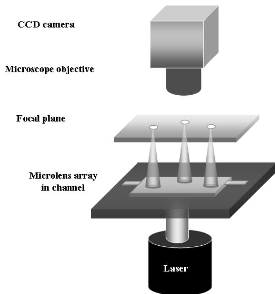
**Figure 5.** Illustration of the instrumentation setup to measure the focal length.
