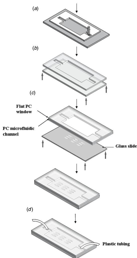
**Figure 3.** The fabrication process of the microfluidic optical device: (a) micromachine the polycarbonate (PC) conduits and chamber, (b) thermal press two PC plates at 140 °C, (c) (1) flip microfluidic channel upside down, and (2) bind glass slide with microlens arrays with microfluidic channels through double-stick tape at four corners and (d) attach plastic tubings.
