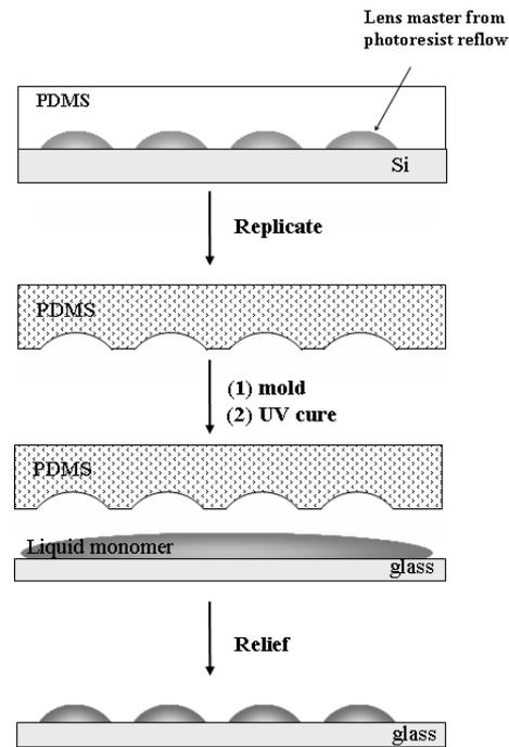
**Figure 1.** The replica molding process to fabricate the microlens array.
