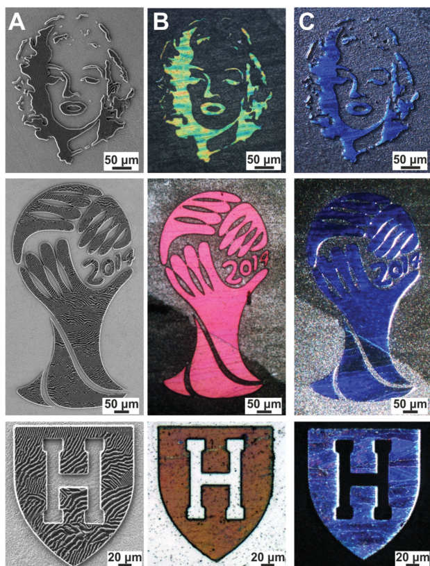
Figure 4. Structural color imaging at micrometer scale. A) SEM images of hierarchical inverse opal structures; microscopy images taken (B) with illumination normal and (C) off-normal to the surface. The images show real, dynamic structural color that blue-shifts with increasing illumination angle.
