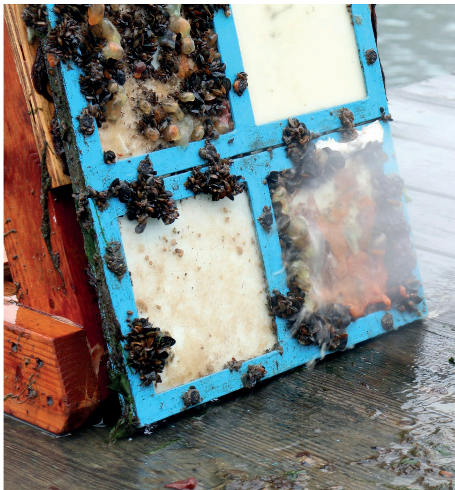
Specially developed paints help to deter marine fouling in field trials.
