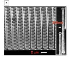
Figure 7. (a) Moving spines and pedicellaria on the surface of a sea urchin; the frame of the micrograph is 5 mm across, while the inset is 100 μm across. (b) Array of synthetic high-aspect-ratio nanospines fabricated in Si that mimic echinoderm skin at the nanometer scale.
